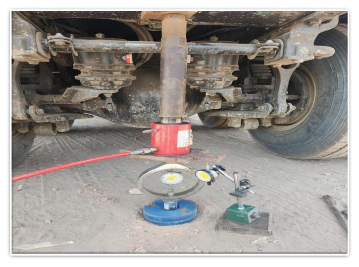
The California Bearing Ratio (CBR) is a measure of the strength of the subgrade of a road or other paved area - IS 2720 (31)
