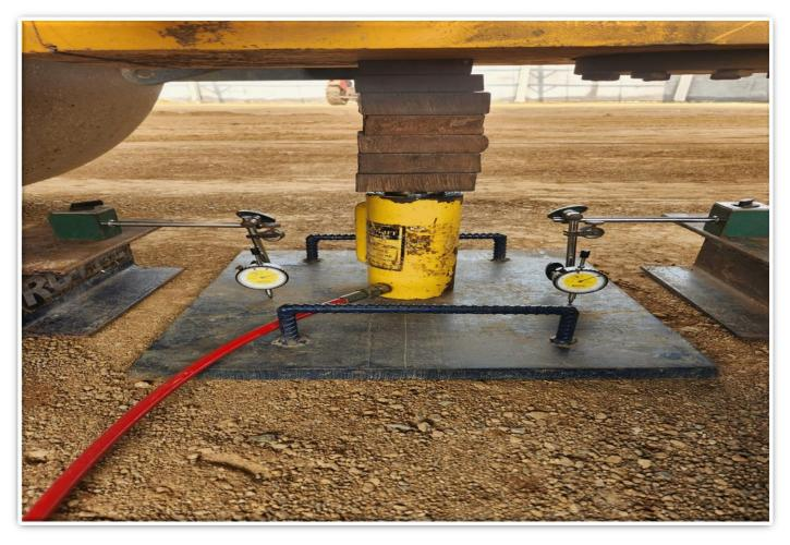
The plate load test is to determine the ultimate bearing capacity of the soil and the probable settlement under a given load – IS 1888
