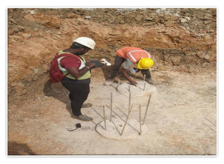
Low strain impact integrity test, is a non-destructive test method for the evaluation of pile quality, and integrity—IS 14893
