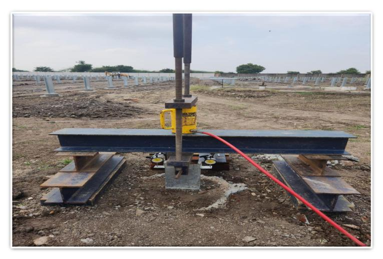
The methodology adopted for Pile Load Test by Pull Out method is in such a way that the hydraulic jack is made to rest on rolled steel joist resting on two supports on the ground – IS 2911 (IV)
