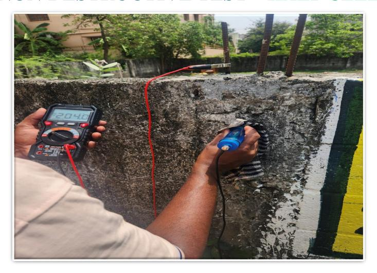
This method may by used to indicate the corrosion activity associated with steel embedded in concrete.—IS 516 (V)
