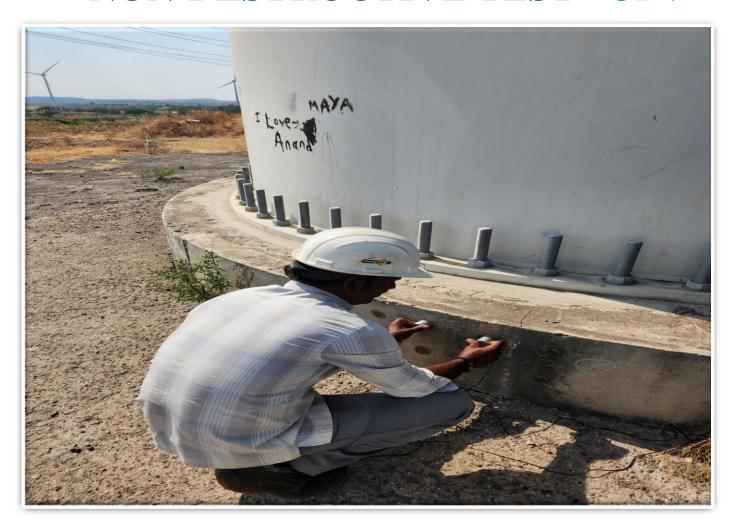
An ultrasonic pulse velocity test is an in-situ, non destructive test to check the quality of concrete and natural rocks - IS 13311
