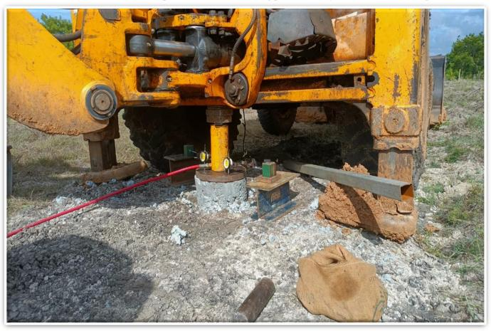
Compression load is applied to the pile top by means of a hydraulic jack using Truck to provide reaction and the settlement is recorded by suitably positioned dial gauges – IS 2911 (IV)
