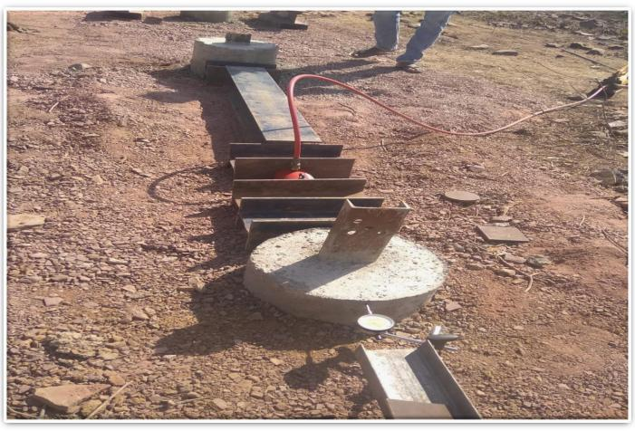
The test is carried out by introducing a hydraulic jack with gauge between two piles or pile groups under test or the reaction may be suitably obtained otherwise - IS 2911 (IV)
