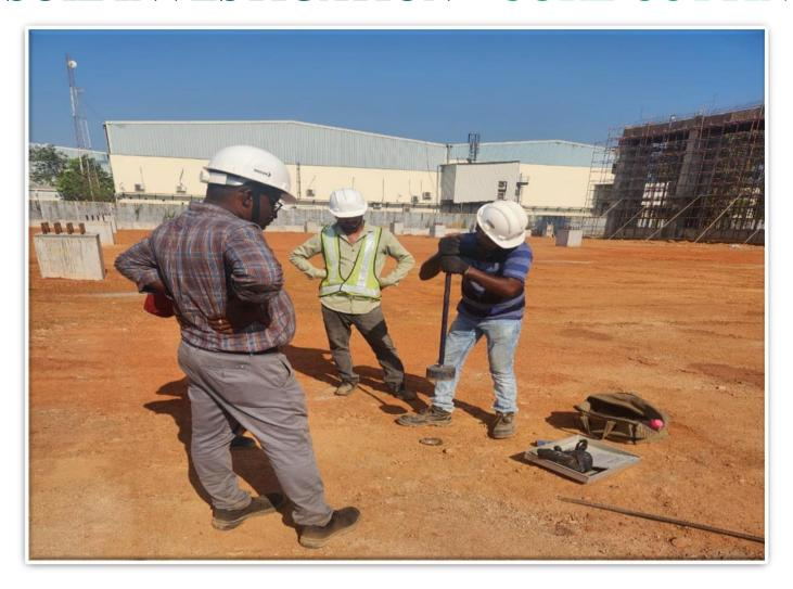
The core cutter method is a test used to determine the in-situ dry density of soil - IS 2720 (29)
