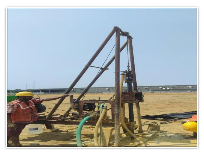
The standard penetration test is an in-situ dynamic penetration test designed to provide information on the geotechnical engineering properties - IS 2131
