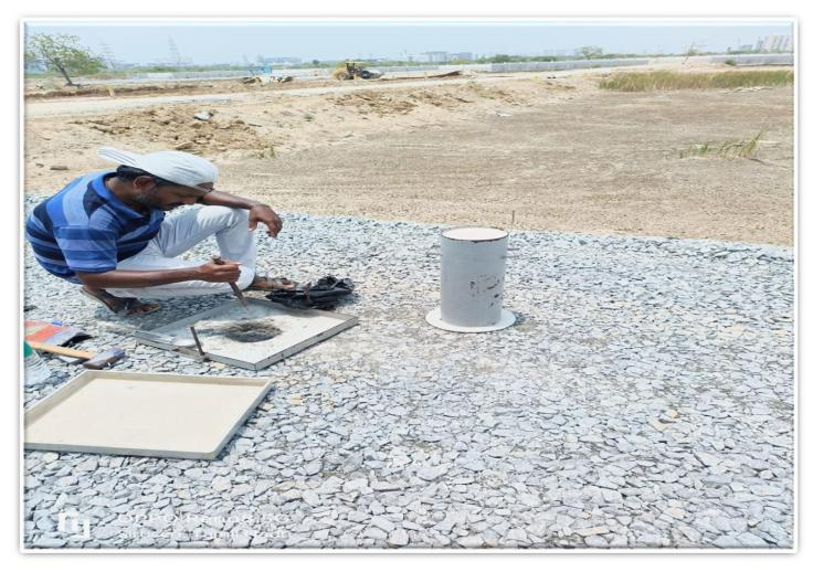
Sand replacement method is used to measure the in-situ density of natural or compacted soils using sand pouring cylinders- IS 2720 (28)
