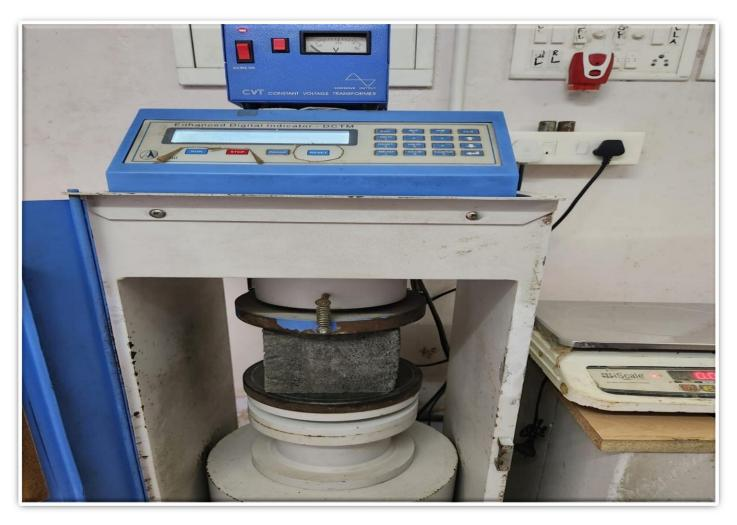
The compressive strength of the concrete cube test provides an idea about all the characteristics of concrete - IS 456
